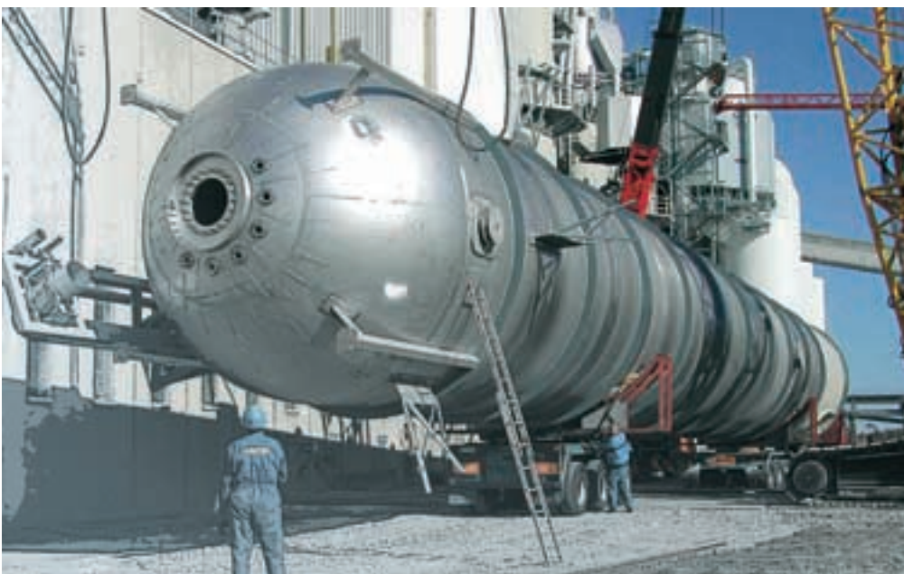
An oxygen/peroxide reactor for bleaching for UPM-Kymmene.
