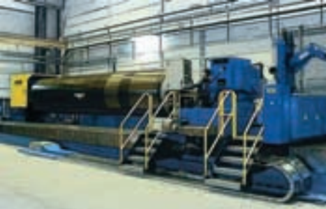
A new CNC turning/grinding machine of AK-Tehdas Oy for rolls up to 80 tons.
