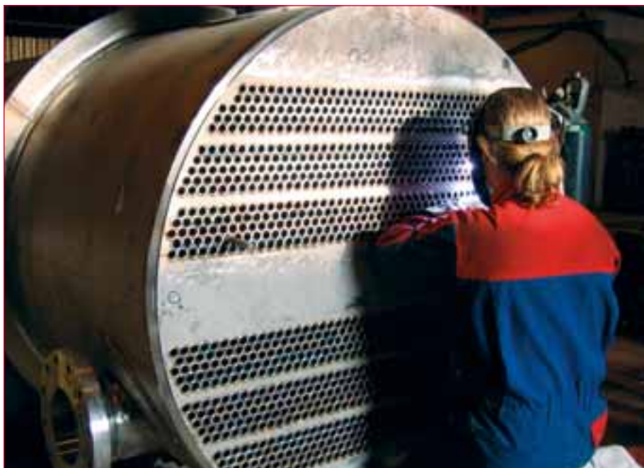
Welding a heat exchanger to be delivered to Sweden for Perstorp.
