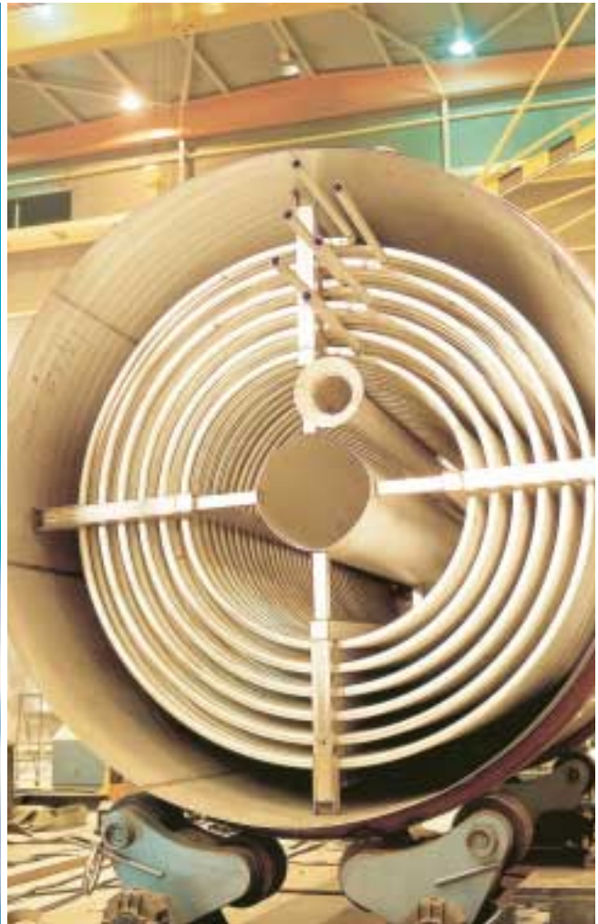
Finnstroi/Riga Penas Kombinat, Pipe coil in ice bank silo
